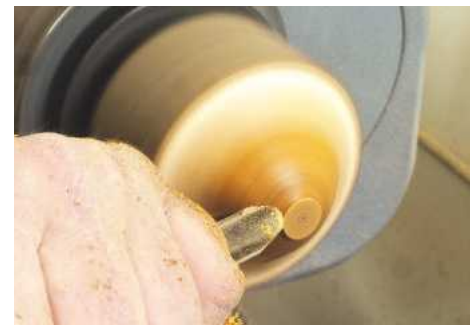
▲ Pic.5 If you do go too quickly you run the risk of pulling a plug of timber from the middle; stopping the lathe and hand sanding across the end is always an option
